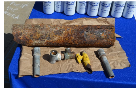
(Above) City of San Diego Mayor Kevin L. Faulconer with SLWA representative, Travis Levers. (Below) Failed water and sewer pipes from San Diego homes.
